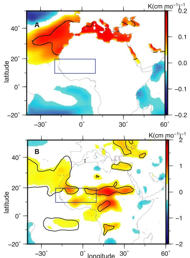
FIG. A4. Regression coefficients [shading,  $\text{K} (\text{cm month}^{-1})^{-1}$ ] for JJA, 1958–2002, for (a) SSTs (ERSST) and (b)  $\theta_{sb}$  (ERA-40) onto West African monsoon precipitation (GHCN), following the removal of the linear variability associated with ENSO. Precipitation was averaged over the boxed region. Black contours delineate regions where the correlation coefficient is statistically significant at the 95% confidence level. Note the different color scales.
