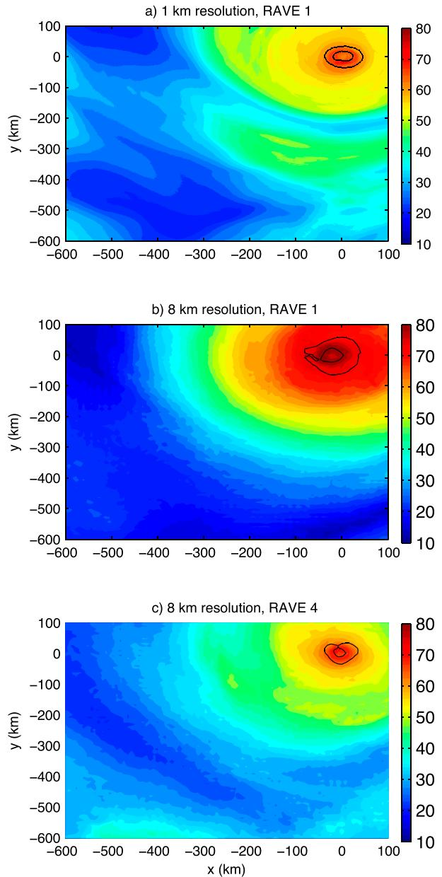
FIG. 11. Precipitable water (mm; color shading) and the  $35 \text{ m s}^{-1}$  surface isotach in rotating domains for different horizontal resolutions on the day when the tropical cyclone first achieves Saffir–Simpson category 2 for (a) 1-km resolution without RAVE, (b) 8-km horizontal resolution without RAVE, and (c) 8-km resolution with  $\gamma = 4$ .
